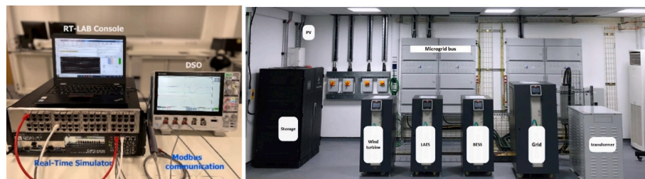
Fig. 11. The real-time hardware-in-the-loop experimental test validations.
