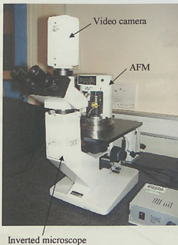
Figure 2-7: Photograph of the combined AFM-inverted microscope.
