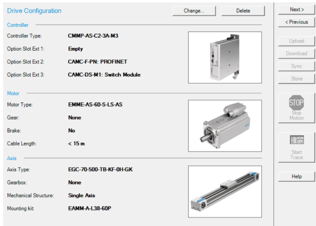
Fig. 7.2: The configuration of drive components in FCT
