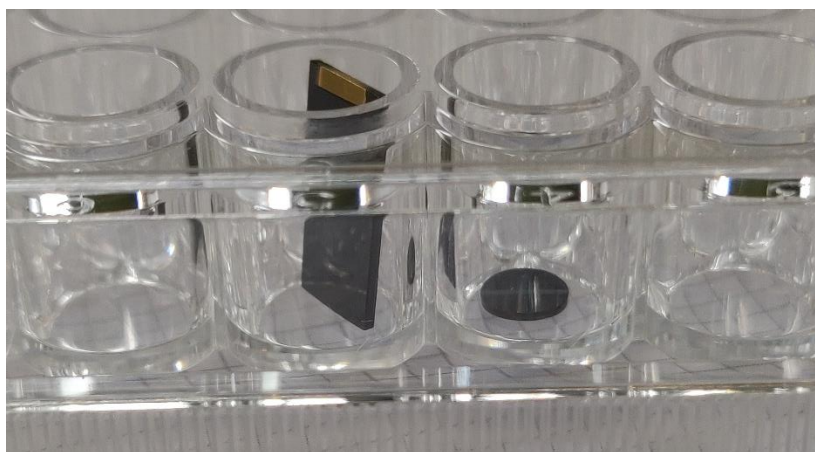
Figure 6.14 Difference between positioning of BDD 4 mm round and 5x10 mm rectangle of BDD in the wells of a 96-well plate for crystal violet assay analysis.
