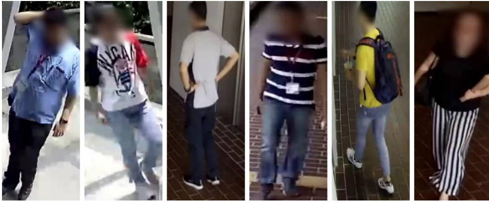
Figure 3.9: Face blurring examples. We apply a Gaussian blur filter to the detected face region to preserve the privacy of individuals in the dataset.
