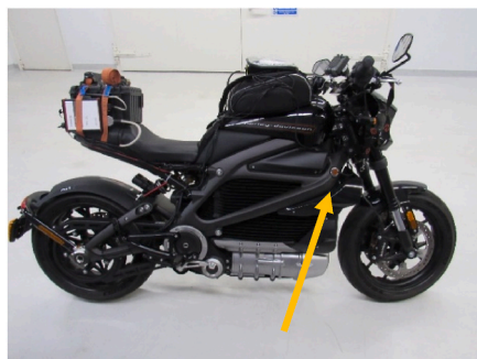
Fig. 3. Harley Davidson Livewire test bike – accelerometer positions highlighted.
