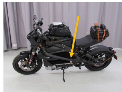
Fig. 3. Harley Davidson Livewire test bike – accelerometer positions highlighted.
