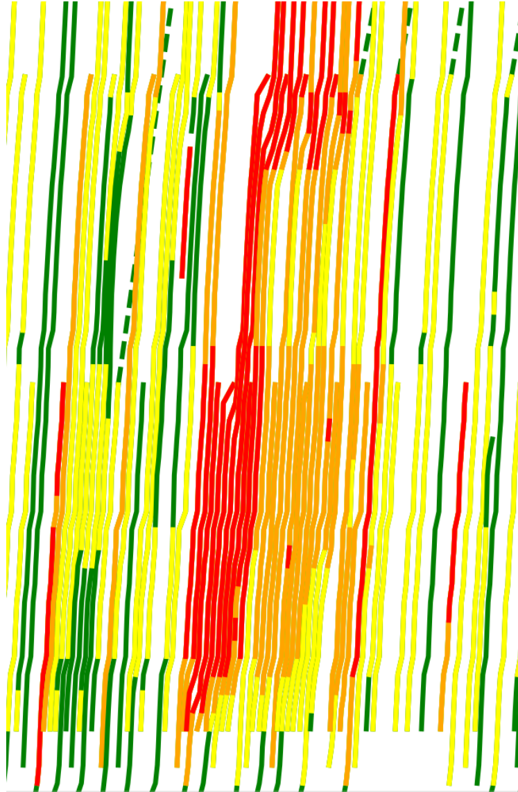
Figure 4.7: Highlighted view of incident in train graph delay format. Trains drawn in green are less than 60 seconds late. Yellow denotes between 60 and 180 seconds late. Orange for delays between 180 and 300 seconds late and red for delays in excess of 300 seconds.
