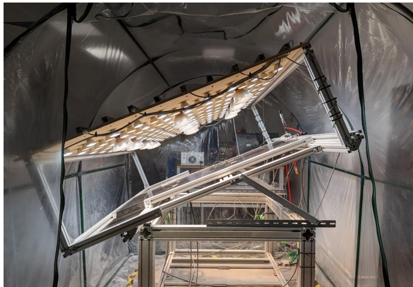
Figure 5-2. Inclined PV-CAES test rig viewed from the side
