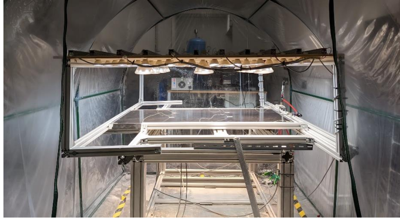
Figure 5-1. Uninclined PV-CAES test rig viewed from the side
