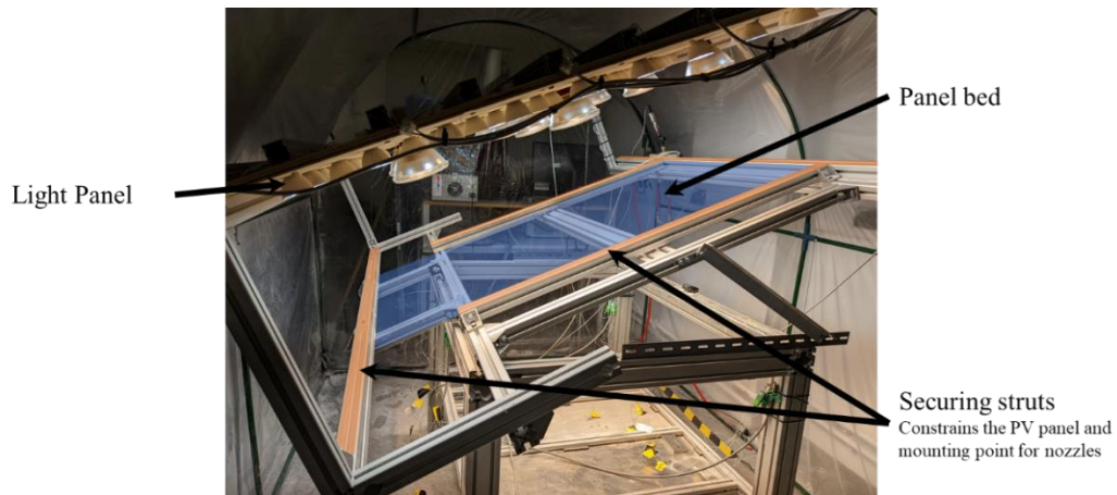
Figure 5-3. Highlight of panel bed and securing struts in the test rig
