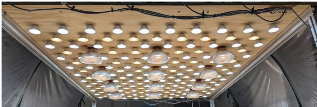
Figure 5-6. Light panel in the test rig
