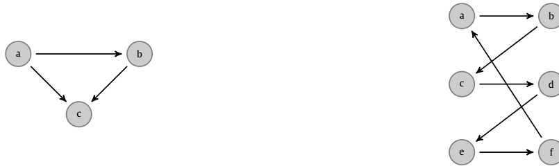
Fig. 5. A non-strategyproof assignment (Left) and a strategyproof one (Right). Algorithm 2 only returns the latter type.
