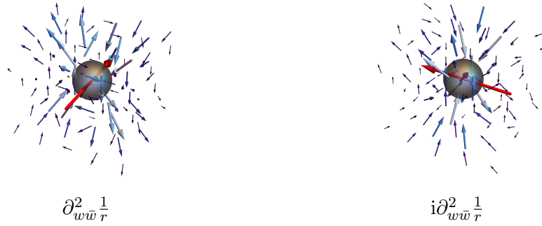
Figure 3.4: Additional flow solutions induced by spin-1 nematic multipoles. The nematic multipoles which induce the flows are shown below them as complex derivatives of 1/r . The red arrows indicate the net active torque.
