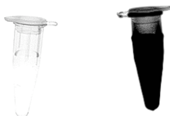
Figure 3.4 Eppendorfs containing ampicillin on the left, and iAmp on the right, visualised in gel imager. Ampicillin and iAmp are visualised on a UV-gel doc. The iAmp sample appears saturated and in this image black, whereas the ampicillin sample does not emit any light at this wavelength so appears transparent.
