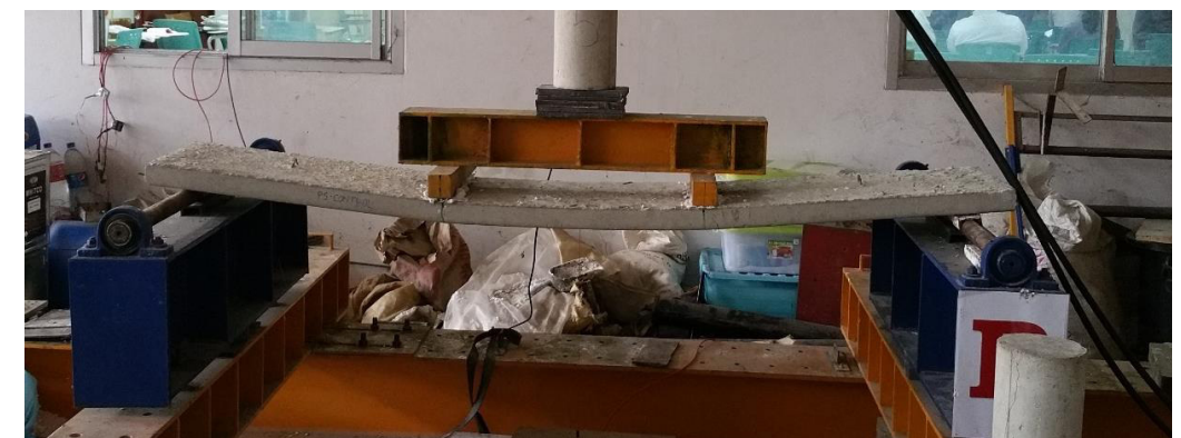
Figure 3. (a) Elevation and (b) cross section of slabs tested in four-point bending and (c) view of slab during test.
