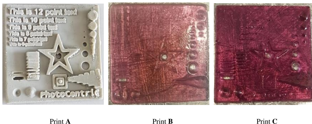
Figure 2.7 - 3D prints of 50:50 w: w TEGDMA 2.5 / UDMA 2.6 utilising thiols 2.11 and 2.12 as co-initiators in blue light, with an exposure time of 300,000 ms. Print B – using thiol 2.11 , Print C – using thiol 2.12 . (Print A – Photocentric standard)
