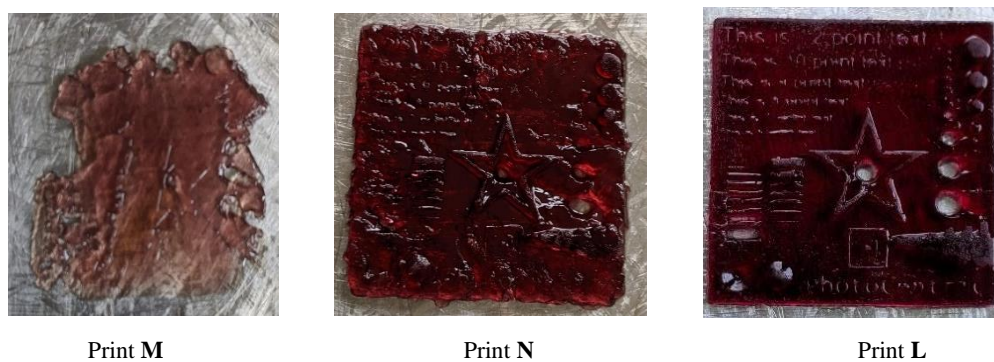
Figure 3.8 - 3D prints using methoxy substituted porphyrins 2.1 , 3.7 and 3.8 as photocatalysts. 2-OMe-TPP 3.8 ( M ), 3-OMeTPP 3.9 ( N ) and 4-OMeTPP ( L )
