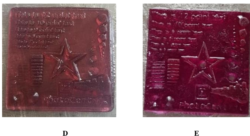
Figure 2.9 - 3D prints of 50:50 w: w TEGDMA 2.5 / UDMA 2.6 utilising thiol 2.12 in blue light, exposure time 300,000ms per layer (Print D ) and 200,000ms per layer (Print E ). (Monomer: thiol: ZnTPP = 200: 10: 0.25)
