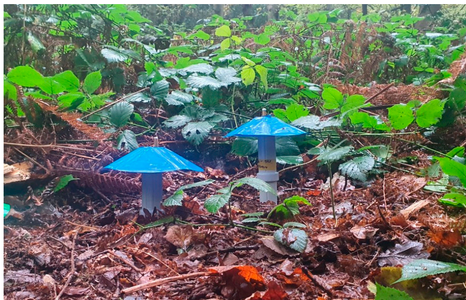
Figure 7. CO 2 probes driven to different soil depths.
