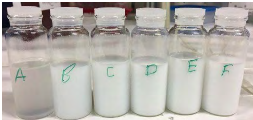
Figure 4.9: Synthesised silica nanoparticles ( \text{SiO}_2 ) with diameter sizes varying from 40nm to 100nm. (A) 45.94nm \pm 2.61, (B) 62.3nm \pm 6.27, (C) 71.98nm \pm 3.42, (D) 86.27nm \pm 4.56, (E) 97.41nm \pm 6.2, (F) 105.04nm \pm 8.63. All samples synthesised by method described previously. (Samples CF-msn-40, through to CF-msn-100). All sample sizes obtained using TEM. The image shows that as the silica nanoparticles get larger a change in colour is observed.
