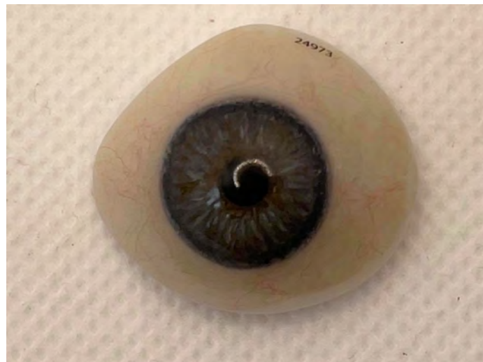
Figure 3.2: Prosthetic eye made using the acrylic polymer Polymethylmethacrylate (PMMA).[12] Image taken 21/08/2021 courtesy of owner.
