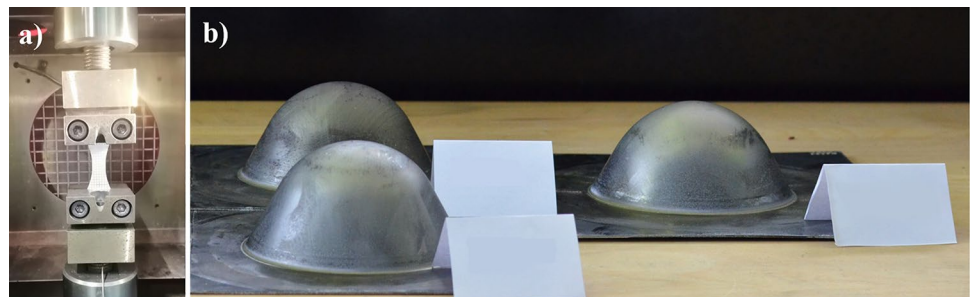
Fig. 1 a) tensile dogbone prior to deformation within integrated load frame furnace, typical gas bulge specimens following failure
