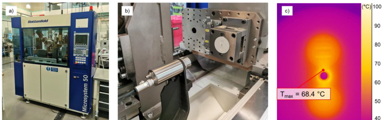
Fig. 2. Images depicting the manufacturing environment and process monitoring approach: a) Battenfeld Microsystem 50 micro-injection moulding machine; b) thermal camera attachment for soft-tool surface temperature measurements; c) a thermal image of the soft-tool showing the maximum temperature (68.4 °C) after ejection.
