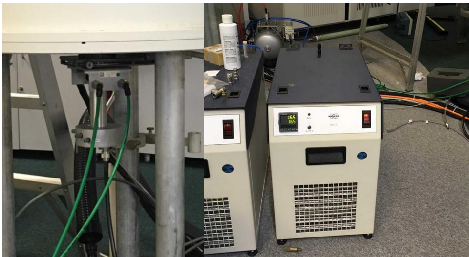
Figure 2.2.8a (left) and (b) right. The cooling mechanism is connected via pipes (a) to the MR probe which it inserted into the underside of the NMR spectrometer. The cooling pump (b) maintains constant temperature of the coolant water at 16.5 degrees Celsius during operation.
