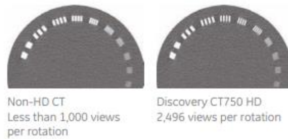
Figure 2.3.6.2.2: Number of views per rotation of the scanner. Figure reproduced from (GE-Healthcare, 2011)
