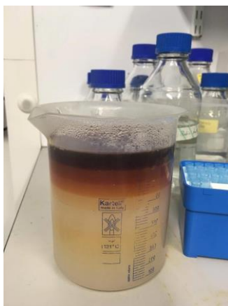
Figure 4.4.1.2.1: Layered agarose gel, with concentrations ranging from 0 to 7681 \mu\text{g}/\text{mL} Iron (III) Chloride
