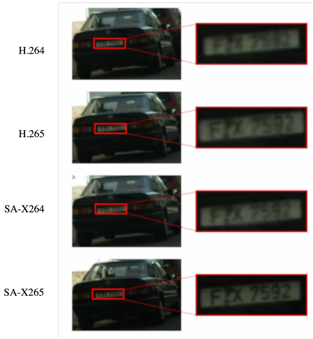
Fig. 8. Visual comparison of a frame compressed with the 4 different techniques (one per row) with equivalent compression ratio. The plate is clearly readable when using the proposed semantic aware compression techniques.
