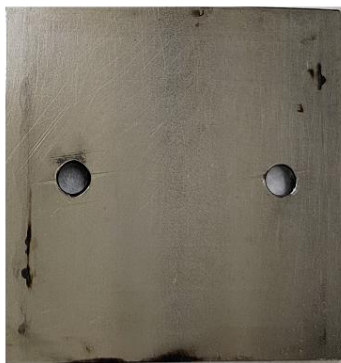
Fig. 7.15. Photo of corrosion displayed on current collector post testing.
