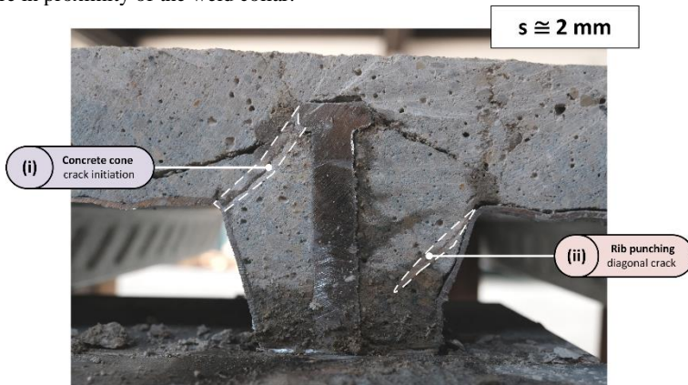
Figure 3. Damage pattern observed after testing at a slip of ca. 2 mm [10].
