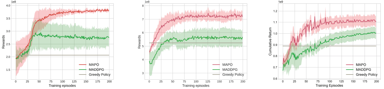
Fig. 8. Comparison of MAPO with MADDPG and the greedy control policy. Left: results of the wind farm composed of three hydrostatic wind turbines; Middle: results of the wind farm composed of six hydrostatic wind turbines. Right: results of the wind farm composed of nine hydrostatic wind turbines. Please see Fig. 7 for the layouts of the three wind farms.
