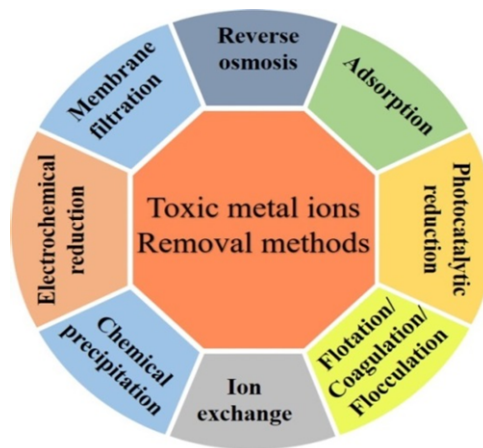
48 49 Figure 1 Different treatment approaches for the removal of heavy metal ions in wastewater (Reprinted 50 from [5] with permission of Elsevier)
