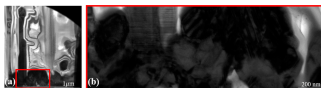
Figure 2. (a) Low- and (b) high-magnification TEM images of the GaAs(P) clusters enclosed in the red square in panel a.
