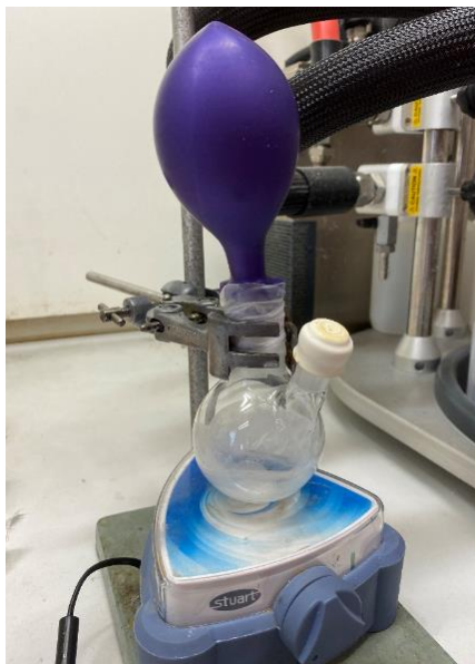
Figure 2.12: An image showing the experimental set-up for the conversions of epoxides to cyclic carbonates using CO 2 . This particular set up is shown at room temperature. Experiments at elevated temperatures were completed in oil baths containing a magnetic stirrer and temperature probe.
