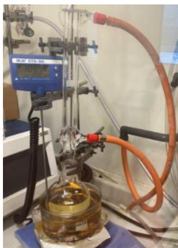
Figure 2.8: An image showing the synthesis of MOFs using reflux conditions.
