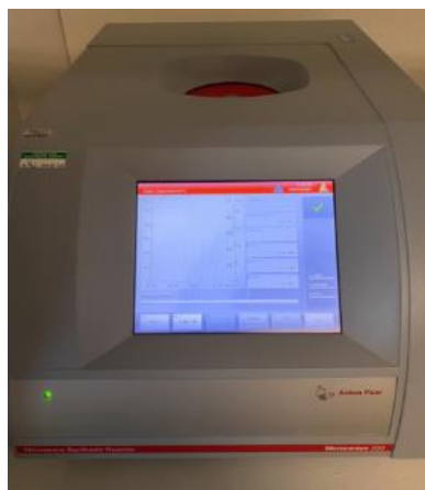
Figure 2.9: An image of the microwave reactor used for synthesis of MOFs.
