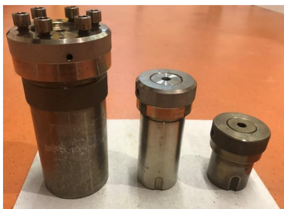
Figure 2.6: An image showing the three different sizes of autoclaves used in this thesis (left-right: 200 mL, 45 mL and 23 mL).
