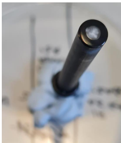
Figure 5.2: An image of the GC electrode with MOF loaded for Mott-Schottky experiments. The MOF coverage was not very homogeneous.
