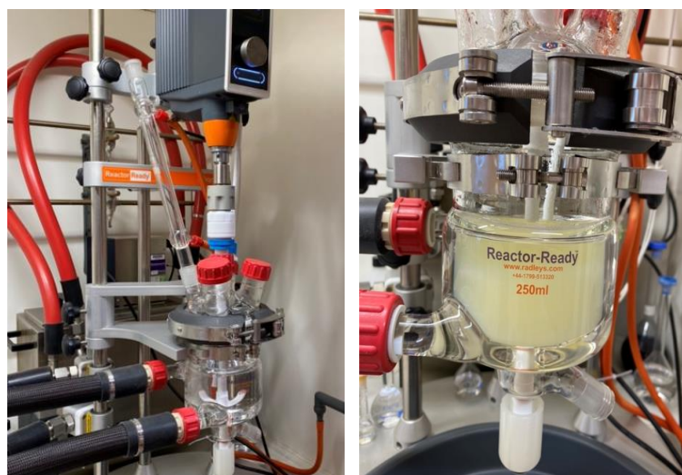
Figure 2.10: An image showing MOF synthesis using a Reactor-Ready™.
