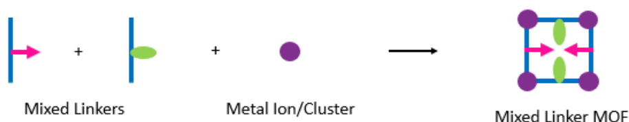
Figure 1.11: A schematic showing the formation of a mixed-linker MOF, reproduced from the literature. 33
