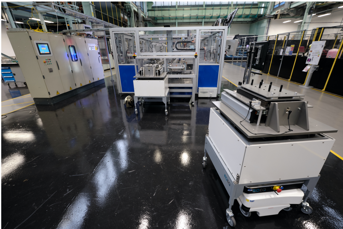
Figure 10. An example material transportation within the IML rig: An AGV is carrying battery cells to the Legacy Loop Assembly Machine in the Stage One where battery modules are assembled.
