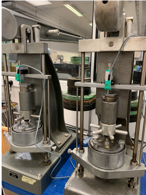
Figure 3.6 - Setup of the standard oedometer tests completed at the University of Warwick.
