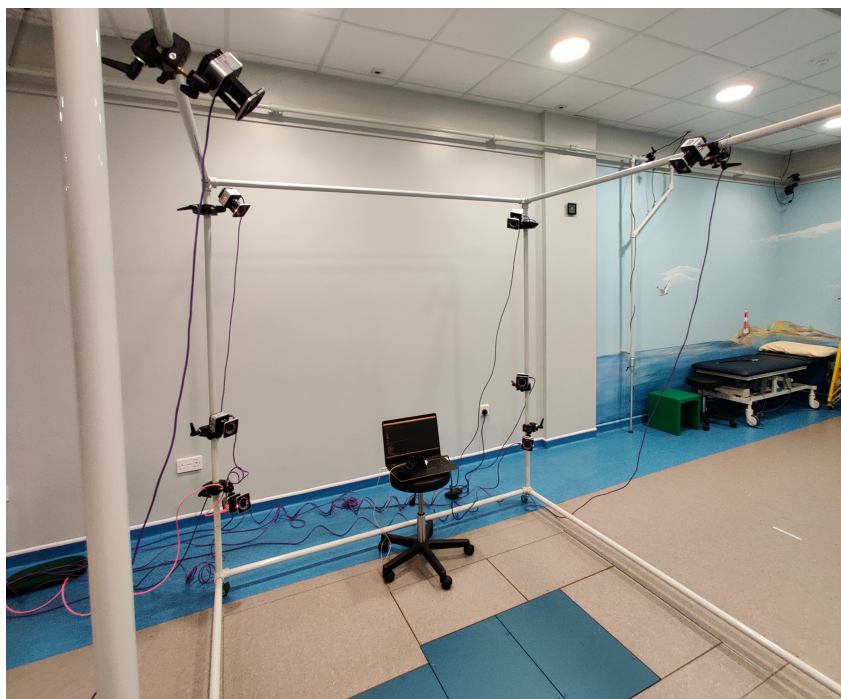
Figure 3.8: The capture space for hand motion capture with a Vicon motion capture system.
