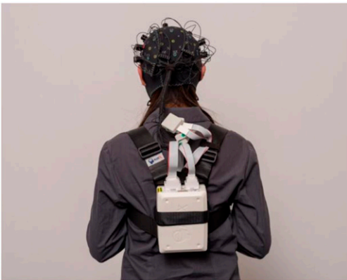
Figure 3. fNIRS equipment. In our experiment, we attached the backpack to the back of the driver's seat. Source: nirx.net .
