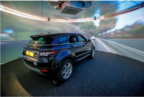
Figure 1. Snapshot of the driving simulator and the virtual environment projected on a curved screen.
