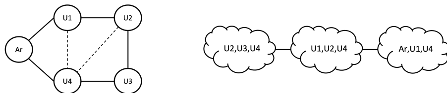
Figure 4.5: a. Triangulated graph for lastFM_cyc b. Junction Tree with three maxcliques of size 3 for the graph
