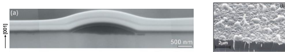
Figure 2.12 a) X-TEM micrograph of a Sn droplet that is formed on the surface of the \text{Ge}_{1-y}\text{Sn}_y epilayer grown on Ge-VS from [87]. b) Scanning electron micrograph of segregation of Sn on the surface of \text{Ge}_{1-y}\text{Sn}_y during epitaxial growth at relatively high temperature of 475\text{ }^\circ\text{C} from [45].
