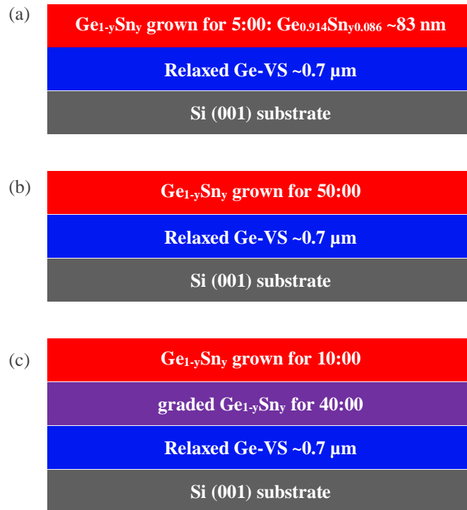
Figure 8.1 Cross sectional schematic of Ge 1-y Sn y as well as graded Ge 1-y Sn y grown on Si (001) substrate via relaxed Ge-VS. All Ge 1-y Sn y layers were grown with the RP-CVD system at 280 °C and 500 Torr using fixed SnCl 4 -H 2 flow rate of 70 sccm. However, for graded Ge 1-y Sn y epilayer, SnCl 4 -H 2 flow rate was tuned from 5 sccm to 70 sccm over its growth time.
