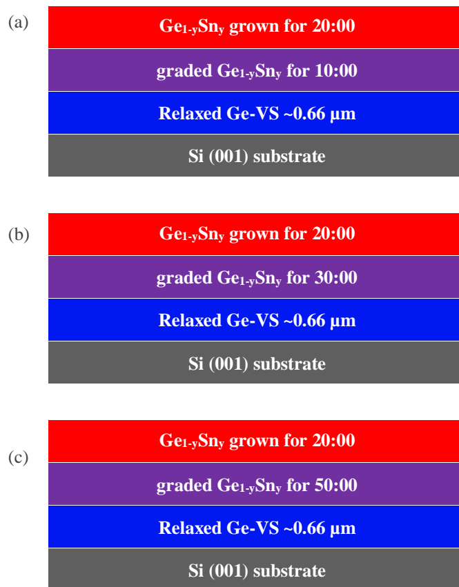
Figure 8.8 Cross sectional schematic of \text{Ge}_{1-y}\text{Sn}_y/\text{Graded-Ge}_{1-y}\text{Sn}_y/\text{Ge-VS}/\text{Si (001)} heterostructures in which \text{Ge}_{1-y}\text{Sn}_y epilayers were all grown at 260^\circ\text{C} and 500 Torr. For the graded \text{Ge}_{1-y}\text{Sn}_y epilayers \text{SnCl}_4\text{-H}_2 flow rate was tuned from 5 sccm to 100 sccm over its growth time of either 10:00 min, 30:00 min or 50:00 min. However, for \text{Ge}_{1-y}\text{Sn}_y epilayers grown on top of the graded ones, a fixed \text{SnCl}_4\text{-H}_2 flow rate of 100 sccm was used over the growth time of 20:00 min.
