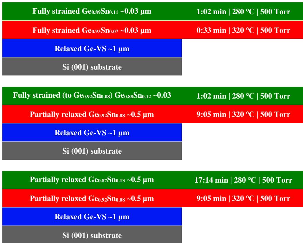
Figure 10.8 Cross sectional schematic diagram of three samples (with different growth time) in which \text{Ge}_{1-y}\text{Sn}_y and \text{Ge}_{1-z}\text{Sn}_z epilayers have different Sn concentration ( y \neq z ) were grown on Si (001) via relaxed Ge-VS. Growth pressure and \text{SnCl}_4\text{-H}_2 gas flow were kept fixed at 500 Torr and 200 sccm, respectively. To achieve two different Sn concentrations, different growth temperatures were used, 280 °C for high Sn concentration \text{Ge}_{1-y}\text{Sn}_y and 320 °C for low Sn concentration \text{Ge}_{1-z}\text{Sn}_z .
