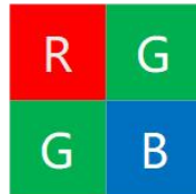
Figure 2. Bayer CFA pattern
