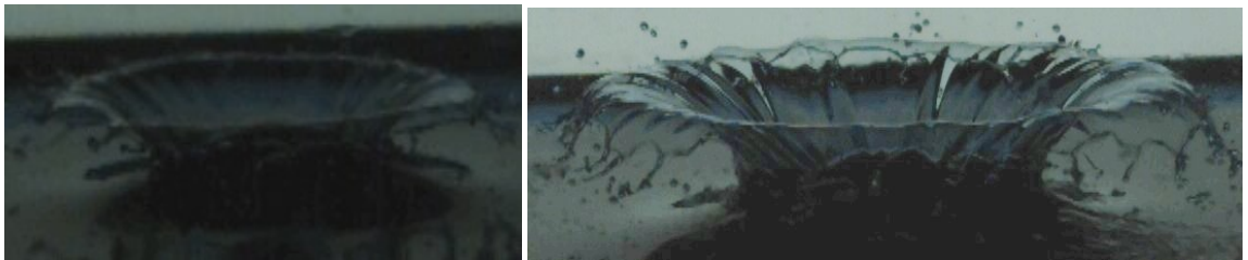
Fig. 4.12 Left: Impact of 8 mm sphere at speed 1.8 \text{ ms}^{-1} in air at atmospheric pressure and liquid viscosity 1.74 cP. Right: Impact of 15 mm sphere at speed 1.8 \text{ ms}^{-1} in air at atmospheric pressure. The similarity of the splash crown at these large sphere sizes suggests that the mechanism for cavity formation does not differ over this range of diameters.
