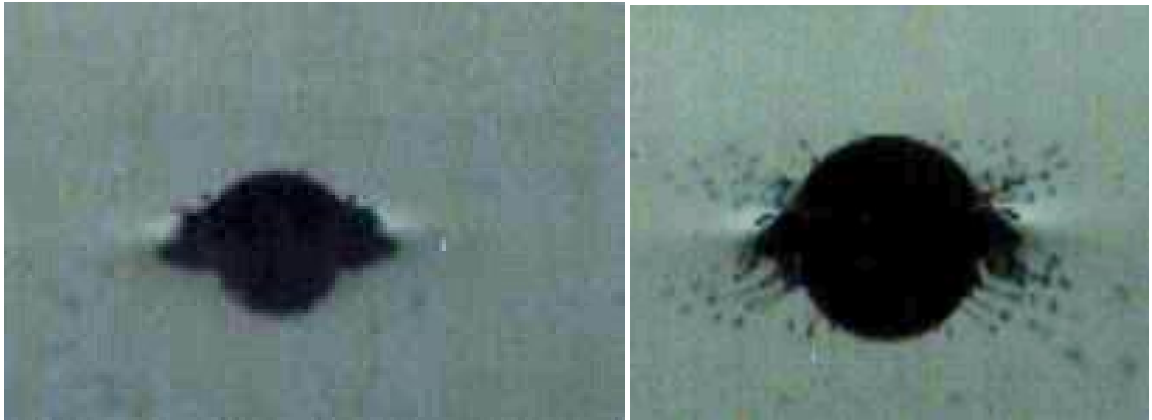
Fig. 4.9 Left: Impact of 2 mm sphere at speed 1.5 \text{ ms}^{-1} in air at atmospheric pressure and liquid viscosity 1.74 cP. Right: Impact of 4 mm sphere at speed 1.5 \text{ ms}^{-1} in air at atmospheric pressure. Although it is difficult to see at such small sphere sizes, it can be observed that the liquid is rising up around the sphere towards the pole.
