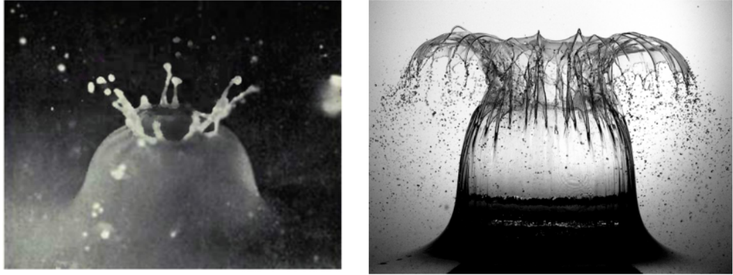
Fig. 1.1 Left: splash created after the impact of a rough sphere on a liquid, obtained using single-spark photography [2]. Right: splash following the impact of a 10 mm steel sphere onto water at 10 \text{ ms}^{-1} at atmospheric conditions, obtained using high-speed photography [3].
