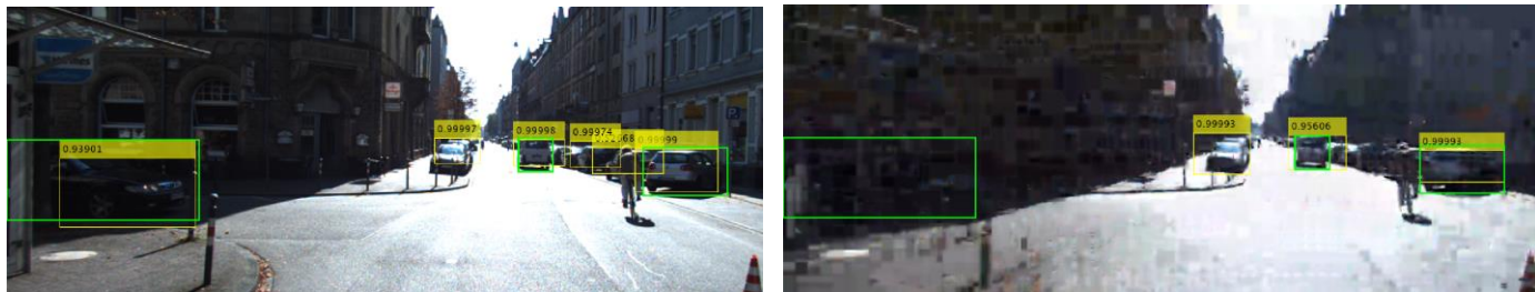
Fig. 5. Sample of the testing dataset with bounding boxes overlaid: green represents the ground truth labels and yellow represents neural network vehicle labels with confidence level above. a) Image compressed at 0 QP with AVC, b) Image compressed at 51 QP with AVC.
