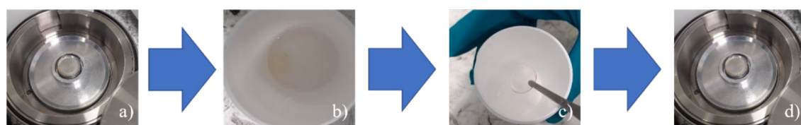
Figure 4. Overview of electrolyte polymer swelling tests. (a) Polymer sample initially dried and weighed, (b) polymer sample immersed in electrolyte for 24 h, (c) polymer sample removed from electrolyte, and (d) polymer samples reweighed.
