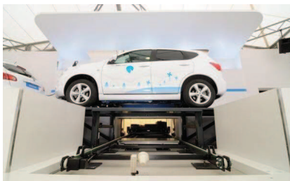
(b) Typical Battery Swapping Operation
