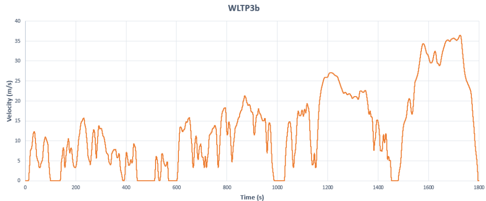
FIGURE 4.5: WLTP 3b drive cycle.
