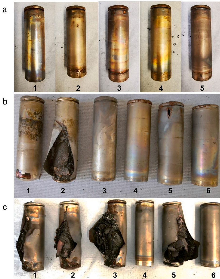
Fig. 4. Photos after test penetrated at different nail diameters. (a) 3 mm, (b) 4 mm and (c) 8 mm.
