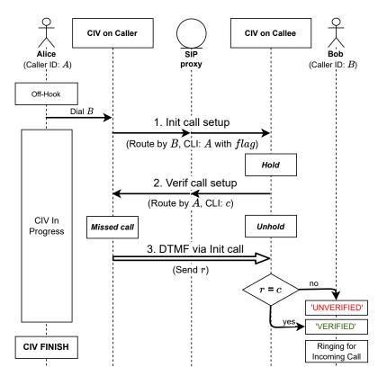
Fig. 7. CIV using CLI/DTMF to send challenge/response
