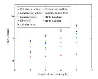
Fig. 12. DTMF transmission time versus number of digits
