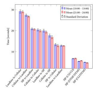
Fig. 9. Delays in CIV between different phones
