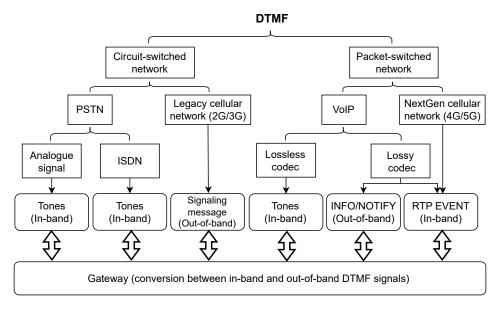
Fig. 1. Overview of DTMF transmission
