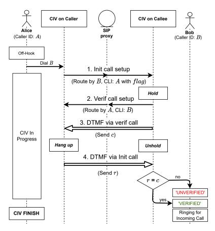
Fig. 8. Using DTMF/DTMF to send challenge/response
