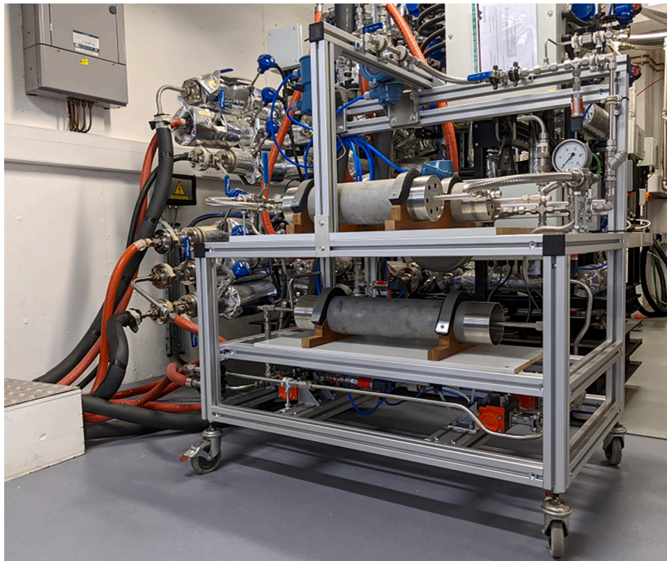
Fig. 22. Image of the proof-of-concept resorption experimental rig in front of the ThermExS thermal test facilities at Warwick, prior to manufacture of the ENG-salt sections and subsequent welding of the reactors.
