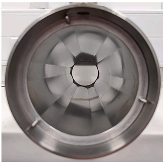
Fig. 17. Front view to the inside of the MnCl_2 HTS reactor prior to assembly. The folded sheet is visible and held in place by two rings at either end of the folded sheet section. The folded sheet aims to minimise heat loss by creating a stagnant ammonia gas layer at the inside face of the shell.
