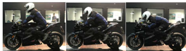
Fig. 1. Rider Positions for Wind Tunnel Testing, from Left to Right; Upright, Mid-position, Tucked-in.
