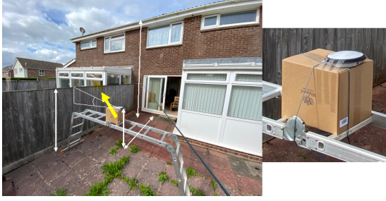
Fig. 1. GNSS receiver placement in a sub-urban environment.
