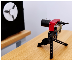
Fig. 9. Prototype of EV-Tach on Raspberry Pi 4B
