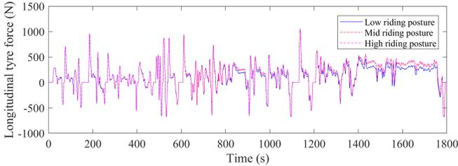
Fig. 6. Required longitudinal tyre force.
