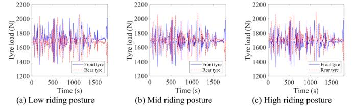
Fig. 9. Tyre load variation under different riding postures.
