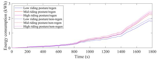
Fig. 5. Effect of riding posture and regenerative braking on motorcycle energy consumption.
