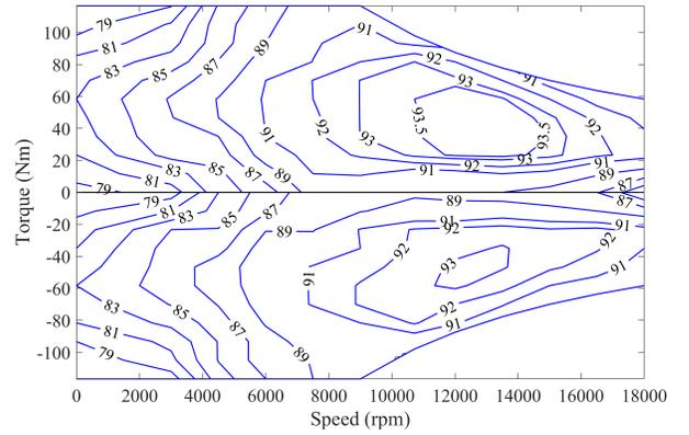
Fig. 1. Electric motor efficiency map (%).
