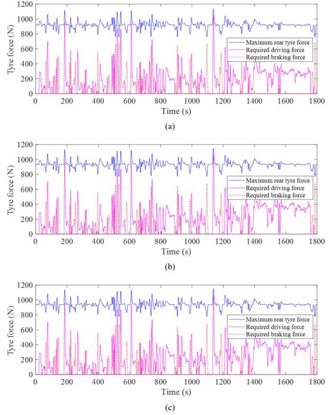
Fig. 12. Maximum rear tyre force and required driving and braking force ( $\mu=0.55$ ), (a) Low riding posture, (b) Mid riding posture, (c) High riding posture.
