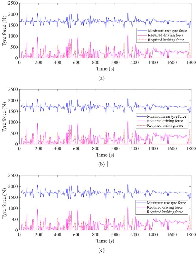
Fig. 10. Maximum rear tyre force and required tyre force ( $\mu=1$ ), (a) Low riding posture, (b) Mid riding posture, (c) High riding posture.
