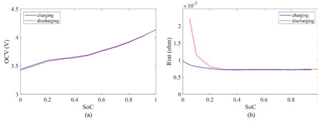
Fig. 2. Battery characteristics. (a) OCV. (b) Internal resistance.
