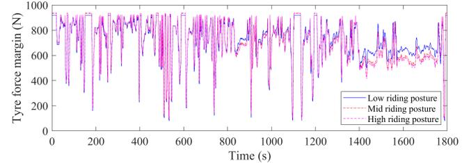
Fig. 13. Rear tyre force margin ( $\mu=0.55$ ).
