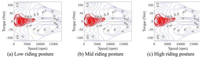
Fig. 8. Motor working points in regenerative braking scenario.
