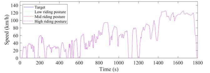
Fig. 4. Motorcycle speed following control for WMTC 3-2.
