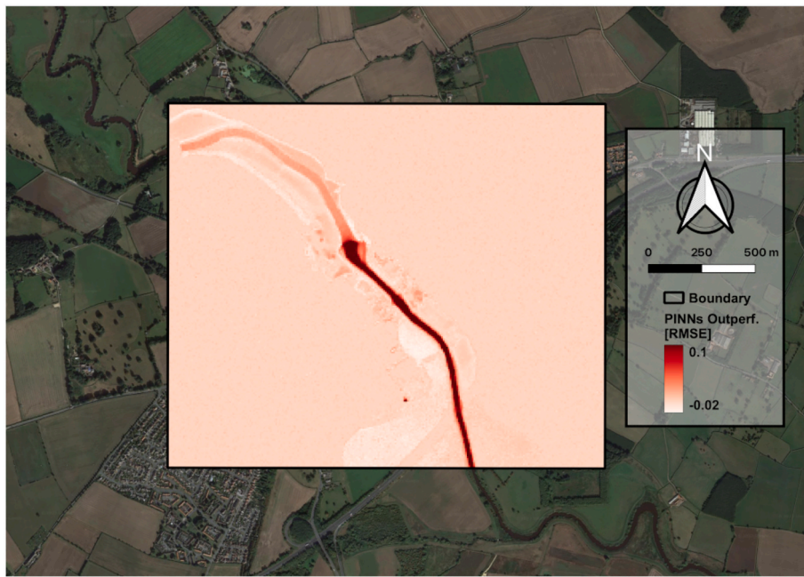
Fig. 9. Illustration of the spatial difference in performance (RMSE) between the CNN model and the PINNs model. Positive values indicate areas where the CNN loss is higher and negative where the PINNs loss is higher.
