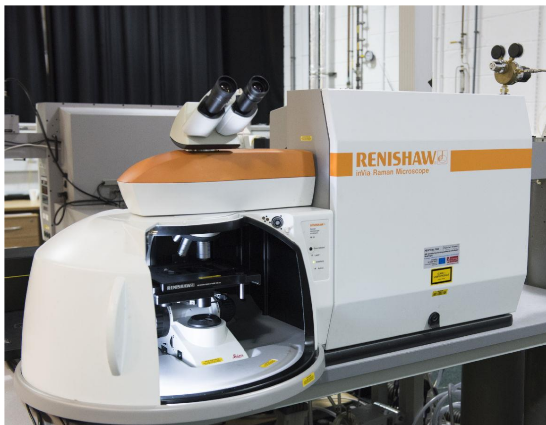
Figure 3.5 – Picture showing the Renishaw inVia spectrometer “Gonzo” with 532 nm laser used to collect some of the data presented in this thesis.
