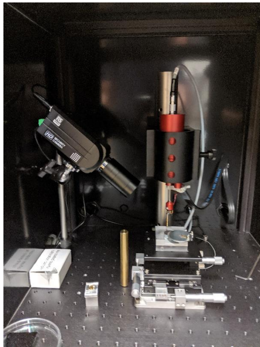
Figure 3.8 – Picture showing internals of the KP Technology KP020 measurement tool
