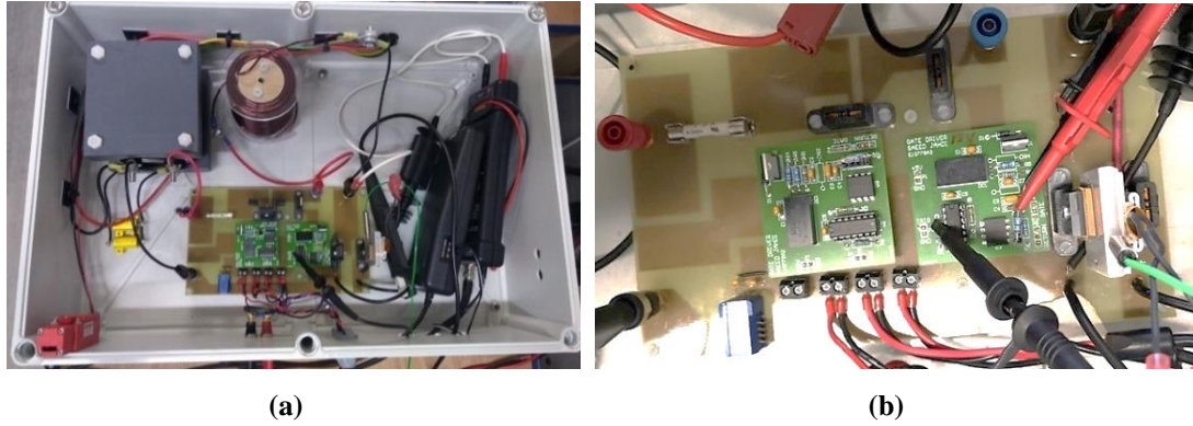
Figure 3.5 (a) Experimental test rig for UIS measurements (b) PCB Board for UIS testing
