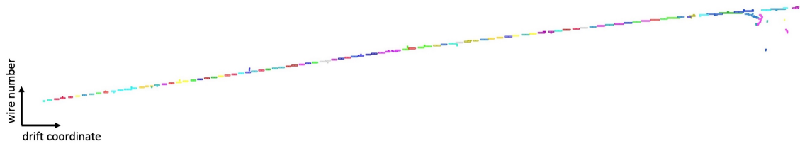
Figure 5.2: The reconstruction of a track that travels parallel to the orientation of the readout wires of one, or several, views. Each colour denotes an individual cluster, some colours may be repeated.
