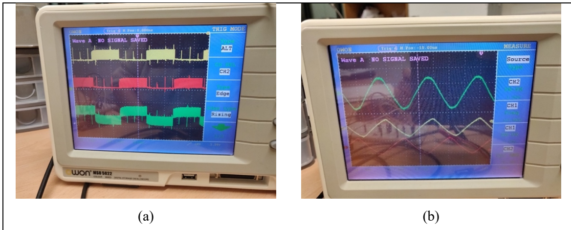
Figure 7.3-11: (a) output from the H-bridge before the Filter, and (b) output of the H-bridge circuit after the filter
