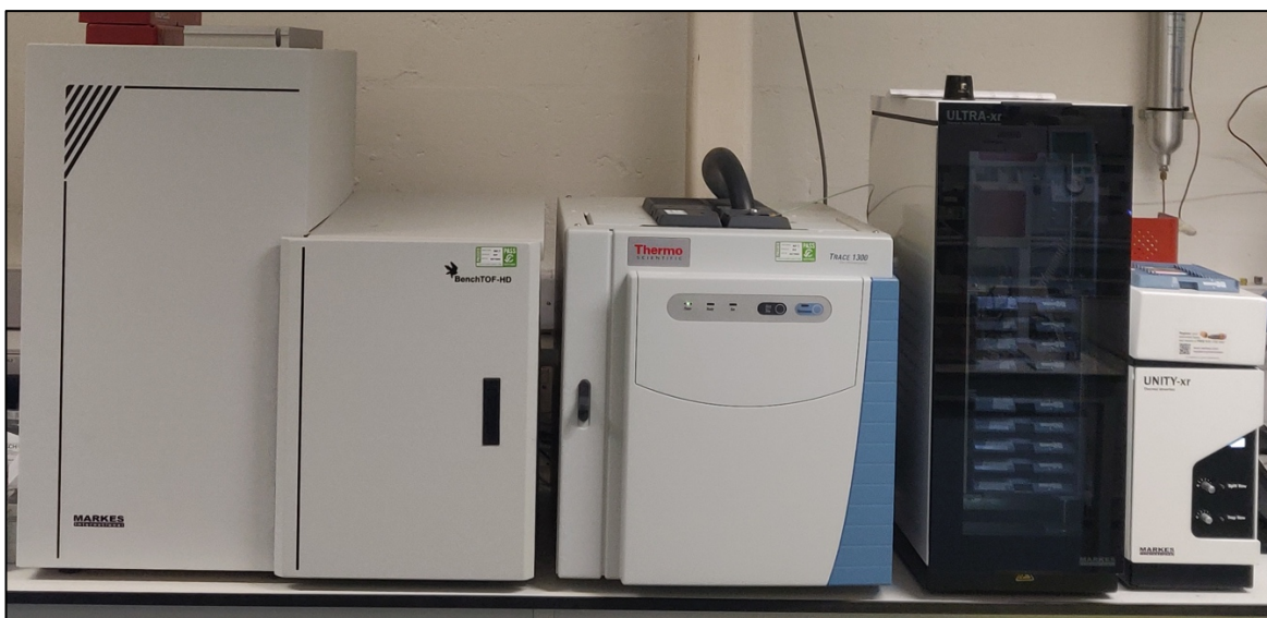
Figure 3.2-1: TRACE 1300 GC - BenchTOF-HD TOF-MS with ULTRA-xr and UNITY-xr
