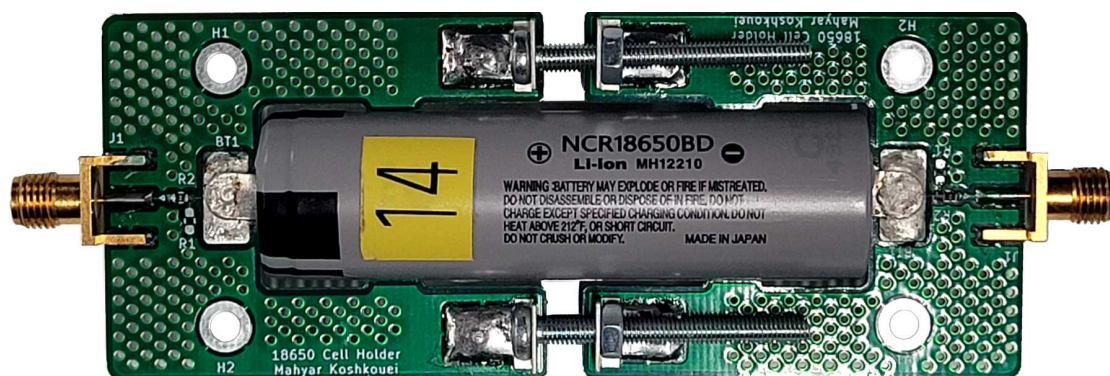
Figure 3.8: The Li-ion cell clamped within the cell holder.
