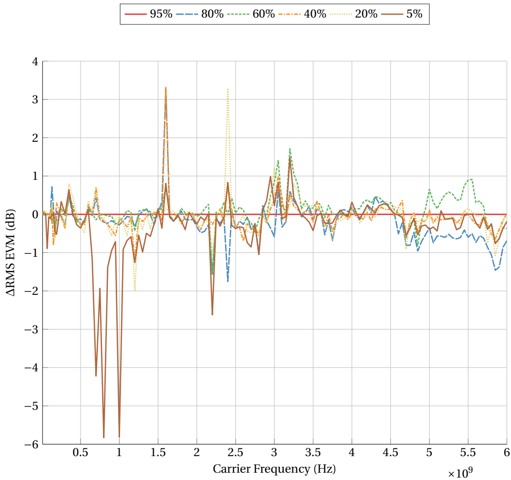
Figure 5.12: Change in RMS EVM of 4-QAM with SoC, using 95 % SoC as a baseline.
